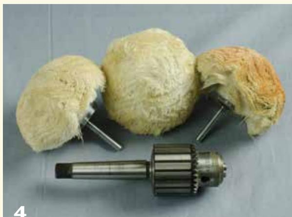
The author's first set of buffs, made of tightly woven cotton cloth. Each buff is mounted in a drill chuck that is inserted into the lathe's headstock spindle.
