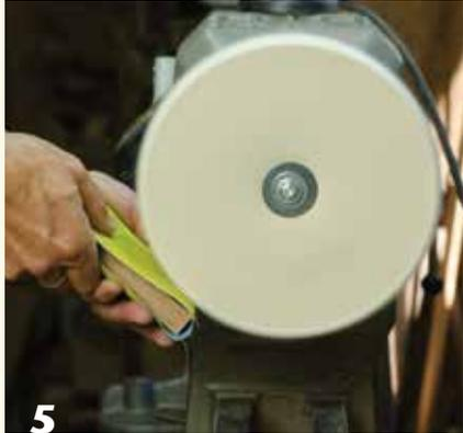
A new wheel will throw off a cloud of lint and should be de-linted before use. This can be done using an abrasive wrapped around a wooden block.
