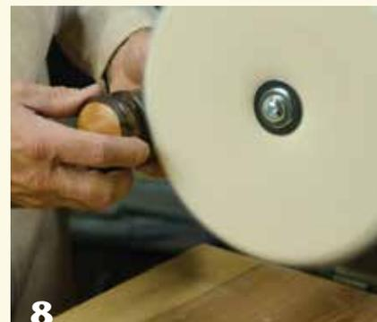
The workpiece should be held tightly to counteract the force of the wheel. Best results are obtained buffing with the grain, as with a handle, but sometimes a piece needs to be presented to the buff without grain alignment to reach between details, such as the beads on this gavel head.
