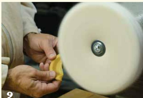
After Tripoli and white diamond, an application of carnauba wax helps protect the final work. Charge the wheel with only a very small amount of carnauba wax.
