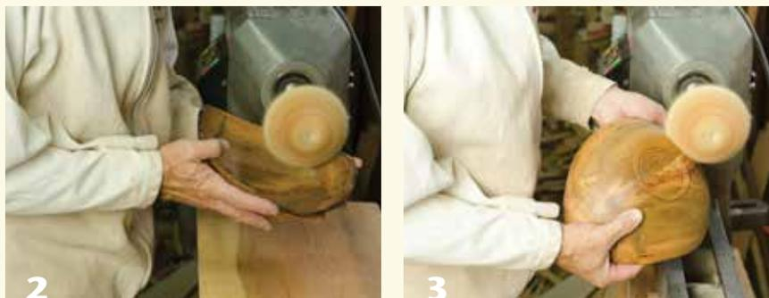
Mushroom buffs can be used on both the inside and outside of an open vessel, making them highly versatile in the turner's shop.
