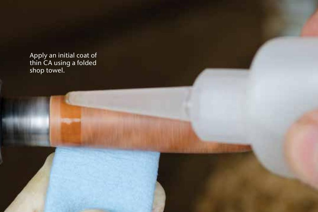
Apply an initial coat of thin CA using a folded shop towel.
