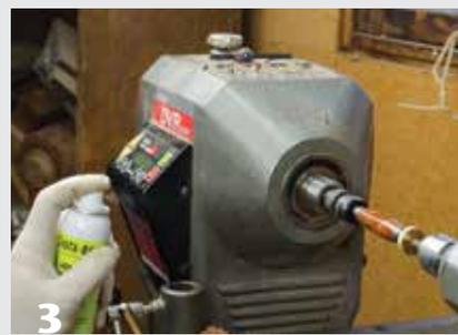
**3** A blast of aerosol accelerator readies the turning for the next coat of CA. Use plenty of ventilation.
