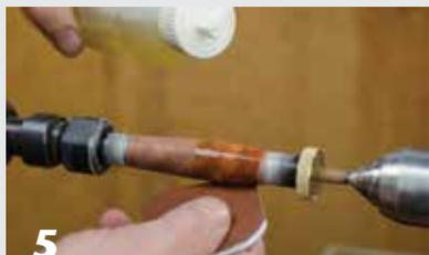
5 Sand with a MicroMesh Polishing Sheet and a few drops of oil for lubrication.
