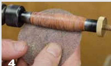
4 Finish the finish with Abranet. The high spots show up as opaque streaks. Aim for a uniformly opaque surface, which is then polished with increasingly finer abrasives.
