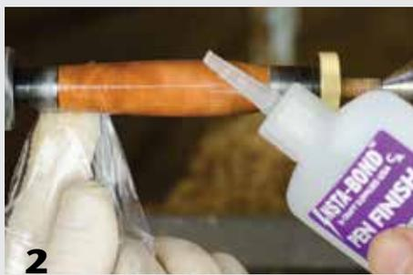
**2** Subsequent applications are with CA that is slower-curing, and a thicker consistency than the first coat, using a plastic-bag-covered finger as an applicator.
