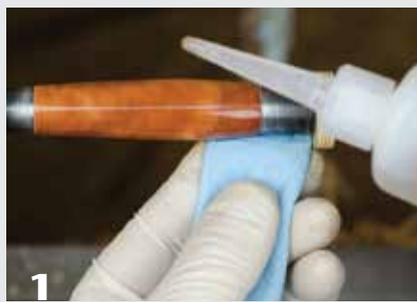
**1** The objective is to apply the CA quickly in a single traverse. CA adheres poorly to metal, so a little contact with the bushings is not a problem.
