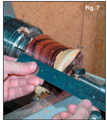
Fig. 7 Measure to predrill a depth hole for hollowing. I like the bottom to have more mass than a typical turning of this dimension, both for stability on the counter and water resistance, so I aim for about 3/8".
