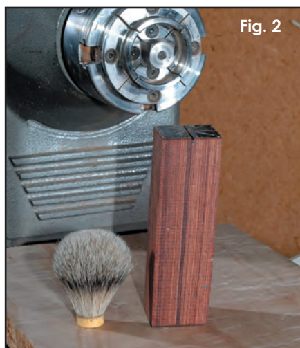
The handle blank is cut to 1-3/4" square x 5", and the brush knot is shown as it arrives in its epoxy plug.
