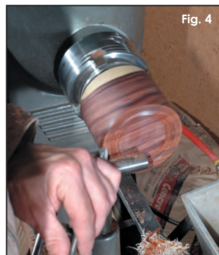
I like to decorate the bottom of the bowl, usually including beads. Make sure to leave enough wood at this point to support expanding dovetail jaws.
