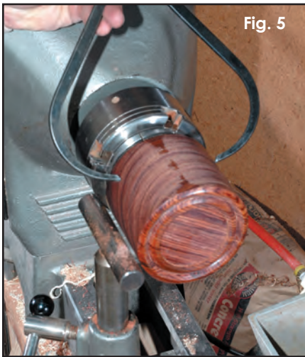
Fig. 5 The appropriate outer diameter of the mug is determined using calipers. Accounting for a 2-3/4" internal opening, this ensures a final wall thickness that will taper out from 1/4".
