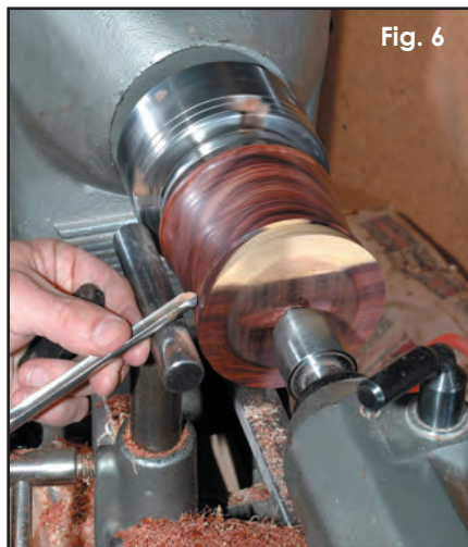
Fig. 6 Final shaping of the outside of the mug includes cutting a bead at the transition point of the external curve.
