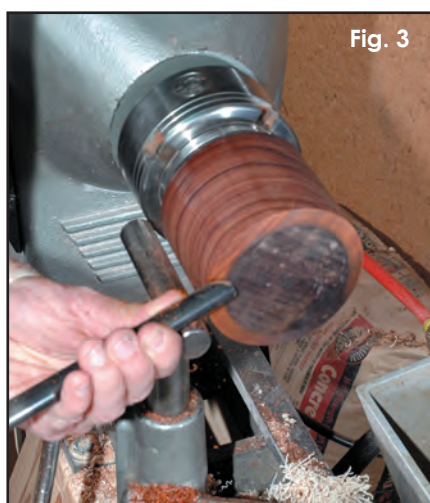
The mug blank is mounted on a screw chuck, turned to round, and the bottom evened out.
