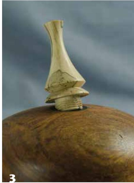
3 This piece of holly had great promise but was so soft from spalting it was a challenge to get an acceptable surface finish. Stabilizing bulked the wood to the point where it would even accept threads.
